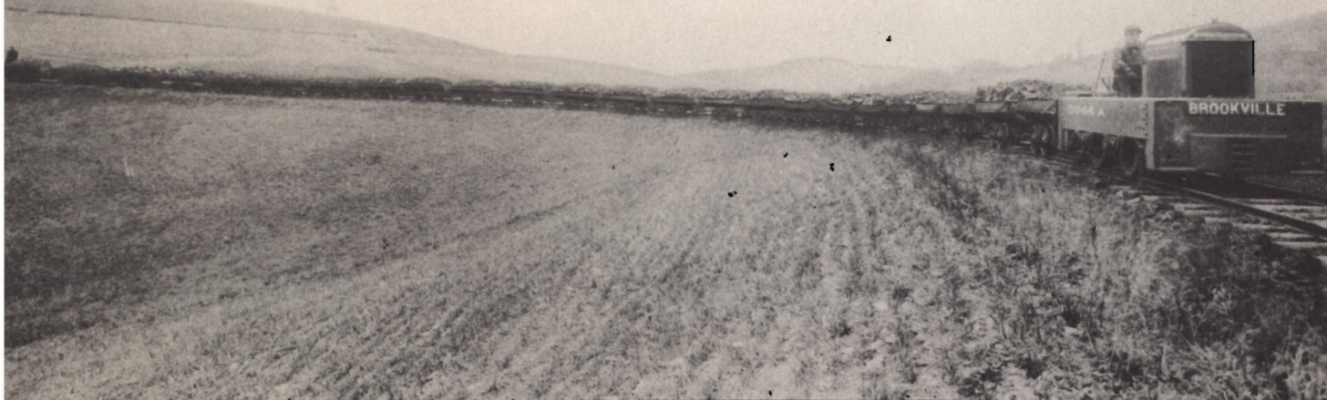
Three-ton 24" gauge International powered Brookville on a sisal plantation.
