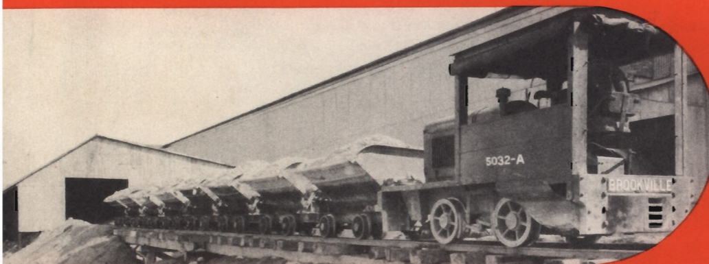
Pulling eight 3-ton cars up a 2% grade at A. P. Green Fire Brick Co.
