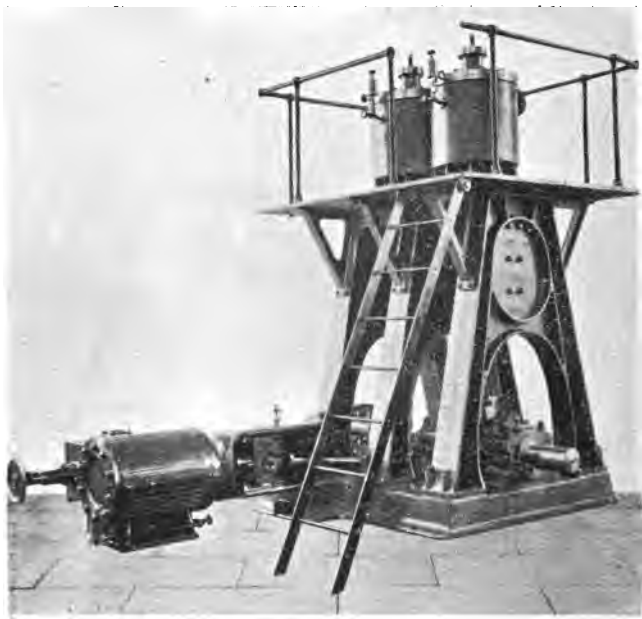
FIG. 48—Class H.—Rix Steam Actuated Vertical Compressor. Manufactured by Fulton Engineering and Shipbuilding Works, San Francisco.
