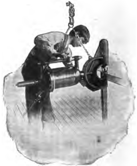
FIG. 12—A PORTABLE PNEUMATIC PUNCH MADE BY MESSRS. F. F. SLOCOMB & CO., WILMINGTON, DEL., U. S. A.
