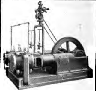
Class F. Steam-driven Two-stage Air Compressor.
