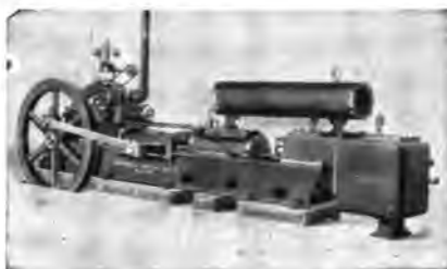
Class "AC 3" 3-Stage Air Compressor.
