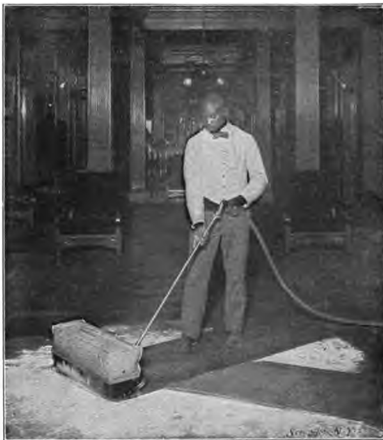
TESTING A RENOVATOR BY REMOVING FLOUR FROM A CARPET. THE DARK STRIPS SHOW THE PORTIONS WHICH HAVE BEEN CLEANED BY THE MACHINE.
