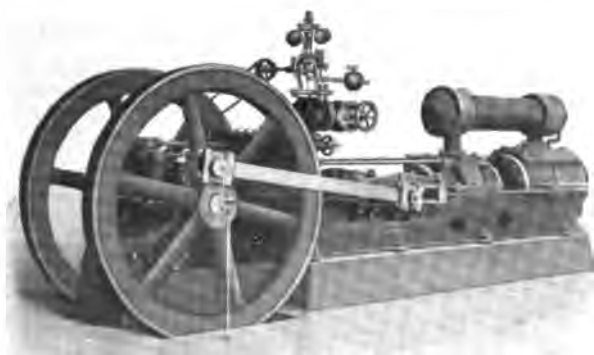
Class "AC" 2-Stage Air Compressor.
