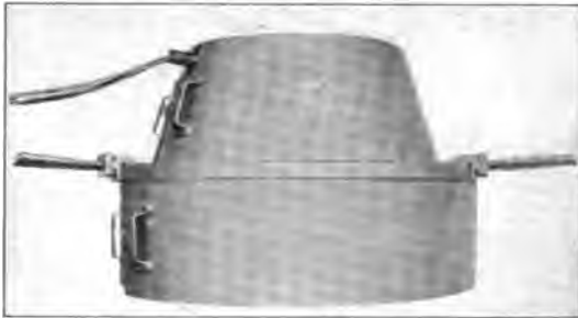
FIG. 3—TURRET CONTROLLER, COVER ON.
