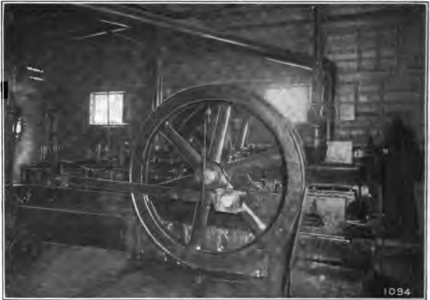
NO. 1—EARLIEST TYPE OF STRAIGHT LINE COMPRESSOR.
