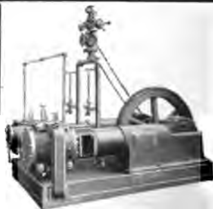
Class F. Steam-driven Two-stage Air Compressor.
