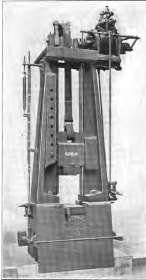
FIG. 1—SIX HUNDRED POUND DROP HAMMER WITH MERRILL-BRETT HAMMER LIFTER.
