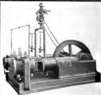
Class F. Steam-driven Two-stage Air Compressor.
