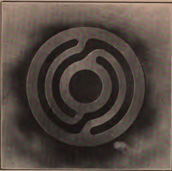
FIG. 57.—Leyner Annular Inlet-Valve
